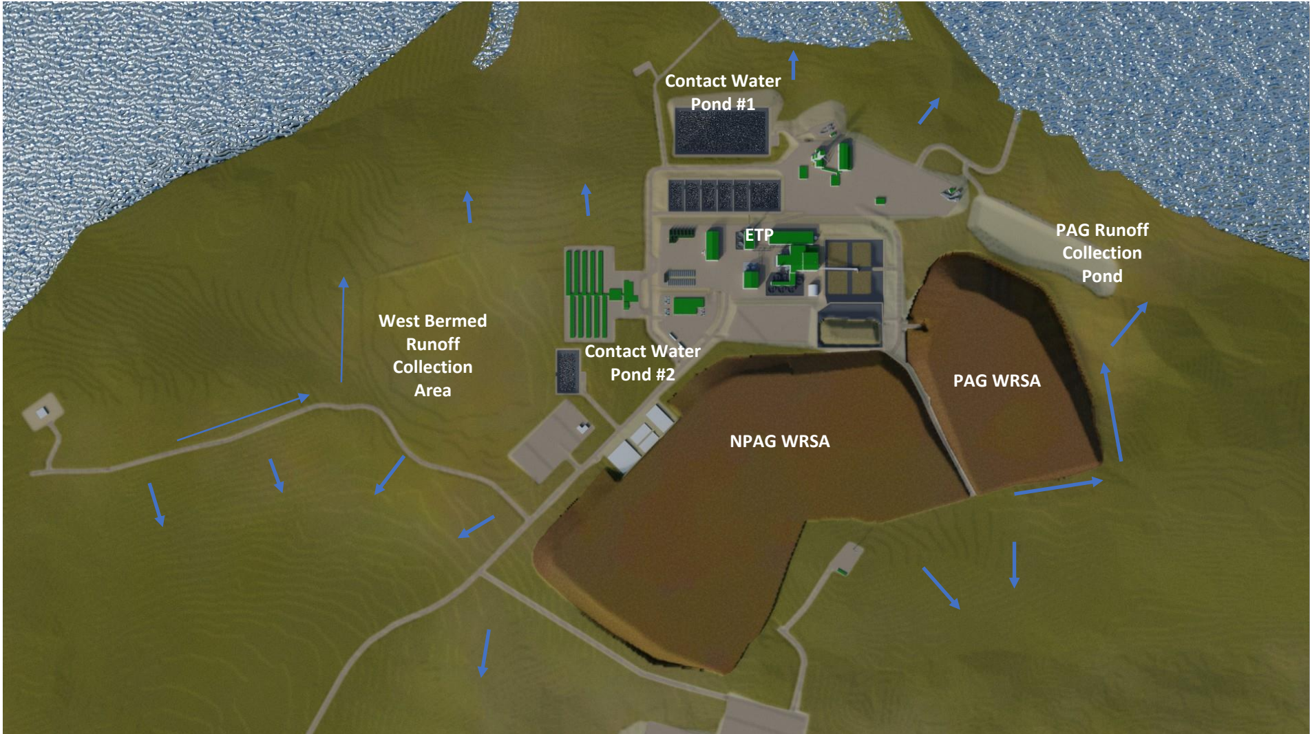
Figure 2: Surface Water Management: Non-Contact Water Diversion (Simplified Diagram)
