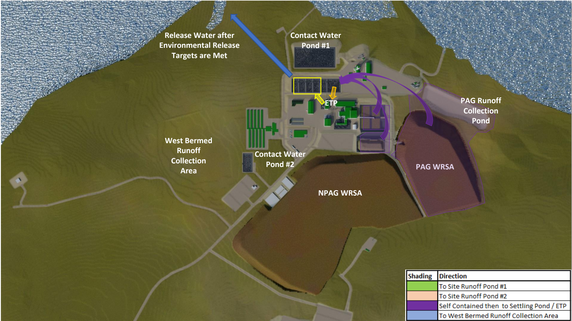
Figure 3: Surface Water Management: Self-Contained Contact Water (Simplified Diagram)
