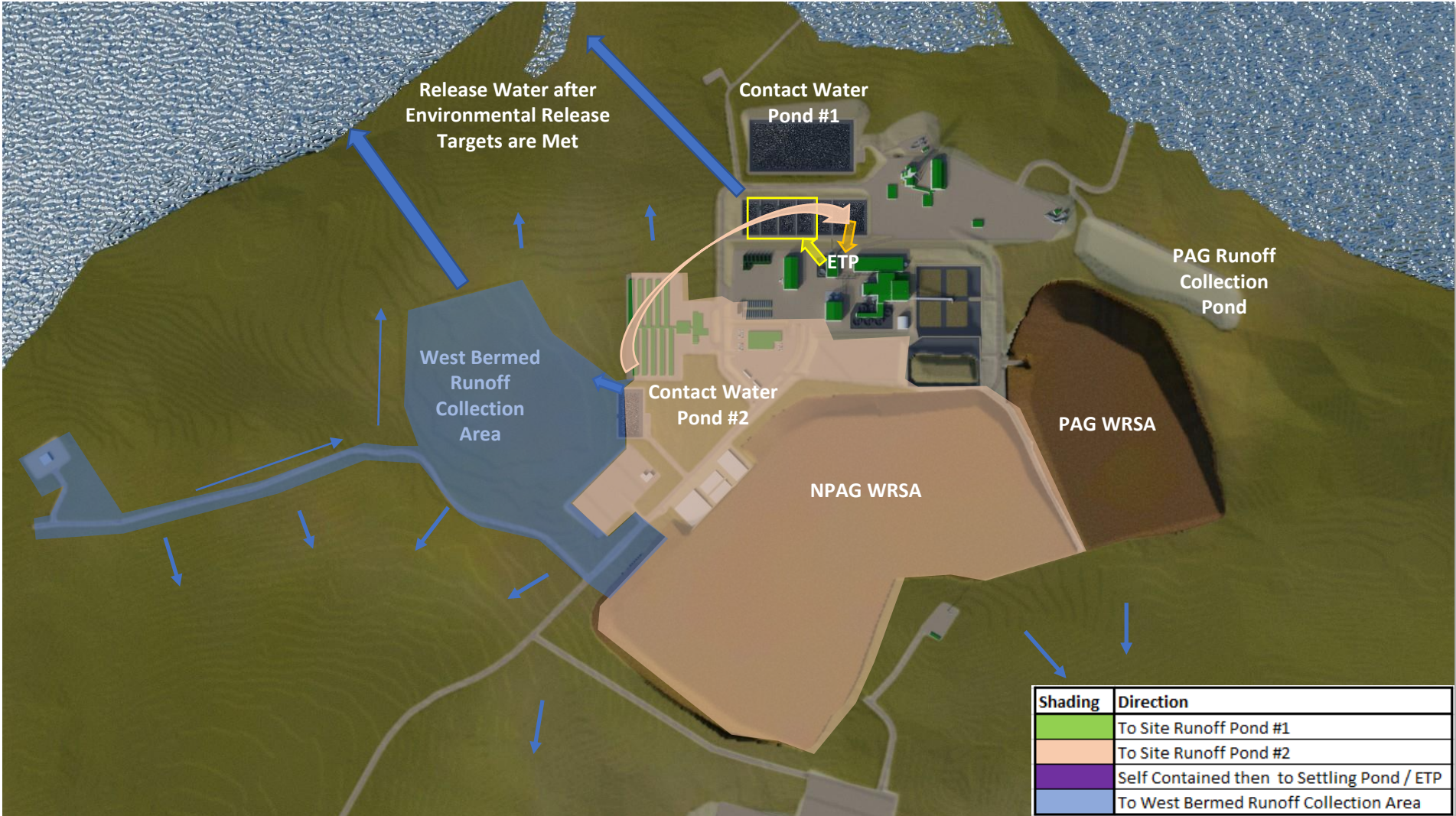
Figure 5: Surface Water Management: Contact Water Pond #2 / West Bermed Runoff Collection Area Drainage (Simplified Diagram)
