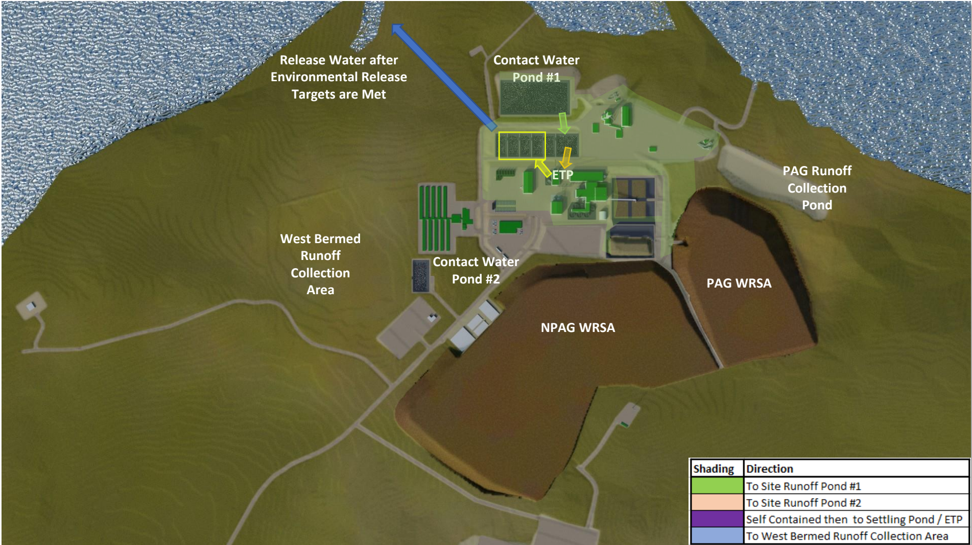
Figure 4: Surface Water Management: Contact Water Pond #1 Drainage (Simplified Diagram)
